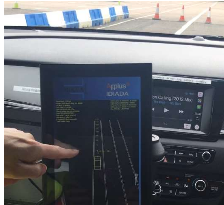
Checking preplotted lane lines against real end of track
