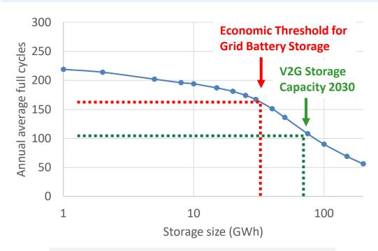
In a grid where supply and demand capacities do not vary, marginal value of deployment reduces.
